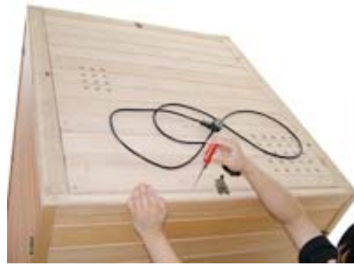
FIG-24 Fix the external board with screws
