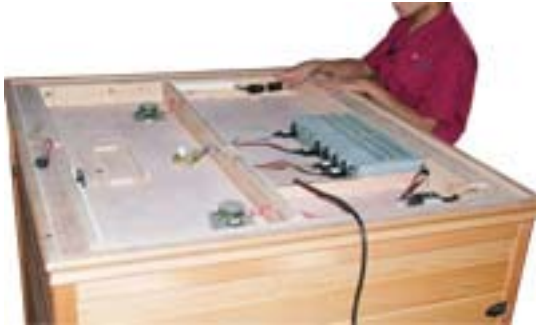
FIG-15 Connectors on the internal top board
