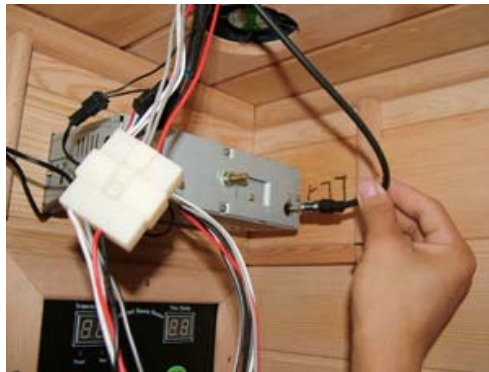
FIG-21 Link the antenna connectors
