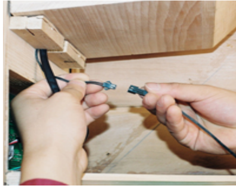
FIG-19 Link the sensor connectors
