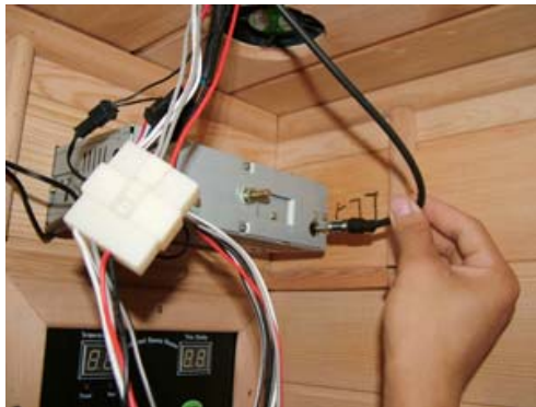
FIG-21 Link the antenna connectors
