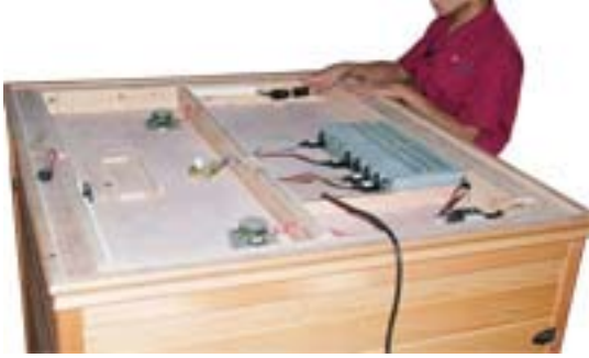
FIG-15 Connectors on the internal top board
