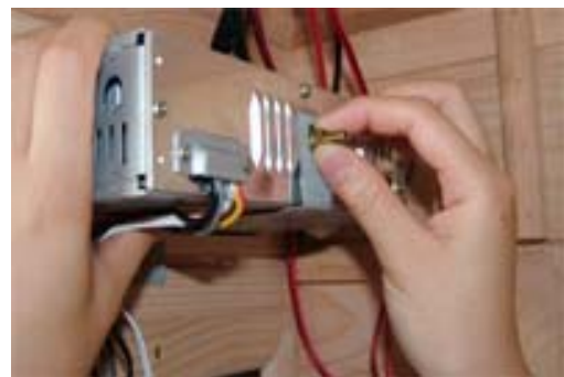
FIG-17.3 Lock the CD with its metal support
