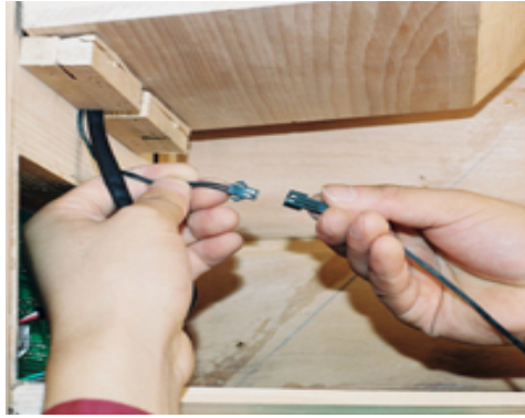
FIG-19 Link the sensor connectors
